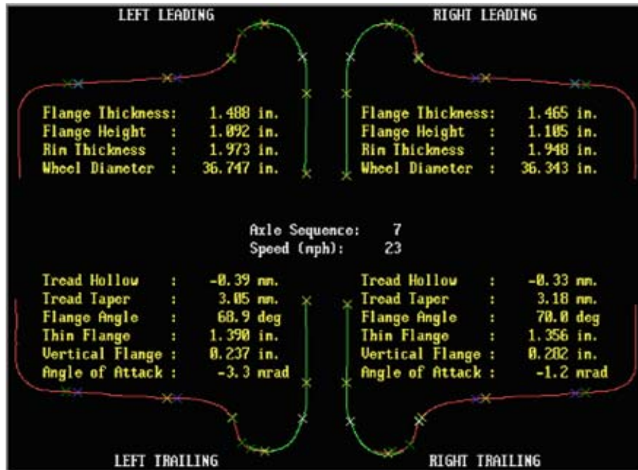
Figure 4 : Profiles of a typical pair of wheels on one axle
